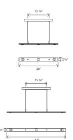
Brevis 42 dimensions - 42" x 2.5" -0.5" H Brevis 28 dimensions - 28" x 2.5" - 0.5 "H [shown] Aluminum Brevis 42 weight - 8 lbs, Brevis 28 weight - 7 lbs Energy efficient LED light source Light output - 1100 lumens [down light - 660, up light - 440] Light color - 2700° K (warm) Color accuracy - 85+ CRI LED power consumption - 16 Watts Dimmable (use ELV or TRIAC dimmer) Ceiling canopy included
